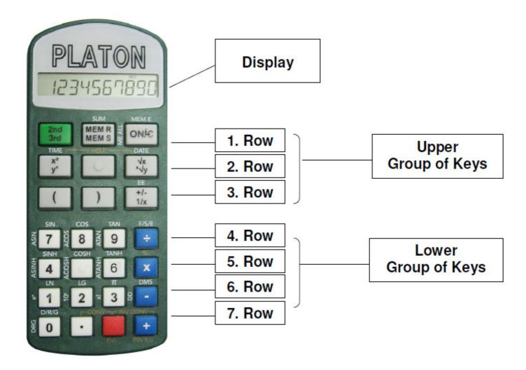
The button in row 1 column 1 has a shift function as known from a PC. A short press activates the second level (layer) of functions connected to the buttons and pressing long activates the third level.
