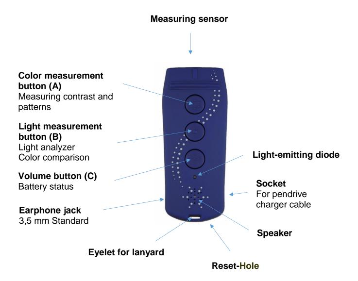
Hold your Color Star device in front of you and in such a way that the control buttons are facing you and the three upper horizontal lines (tactile markings) - above the color measurement button - are directed away from you.
